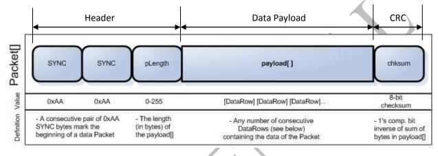
Figure 3. Digital Output Packet Format
