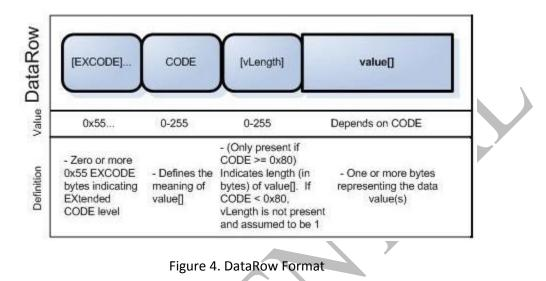
The DataRow may begin with zero or more [EXCODE] (extended code) bytes, which are bytes with the value 0x55. The number of EXCODE bytes indicates the Extended Code Level. The Extended Code Level, in turn, is used in conjunction with the [CODE] byte to determine what type of data this DataRow contains.
